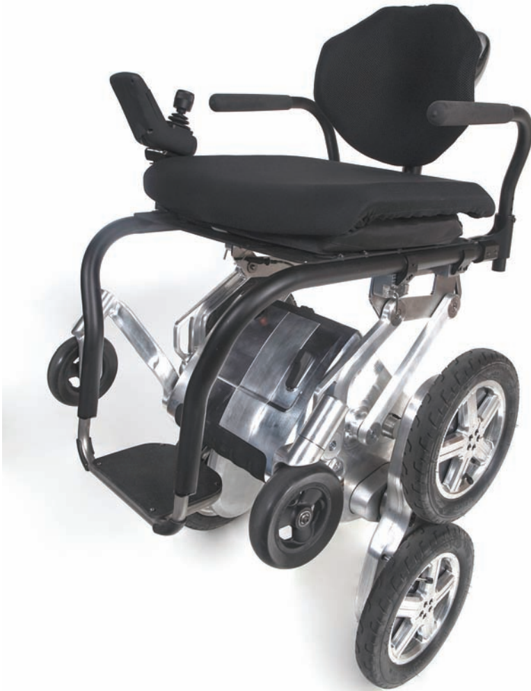
Fig. 4. The iBot Climbing Wheelchair. Toyota Corporation.
