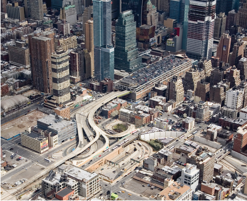
Fig. 10.4. Bus ramps connecting the Port Authority's Lincoln Tunnel with its Midtown Manhattan bus terminal (c. 2006).
