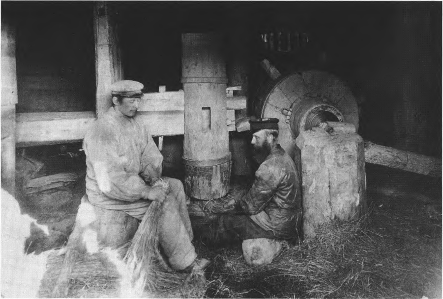
Two men braking flax in a water-powered flax mill. Photo Hälsinglands Museum, Sweden.
