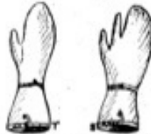
FIG. 2.—Two-fingered glove or mitt, a double-glove. The strap at the wrist is of canvas or rubber; the upper strap is of canvas.
