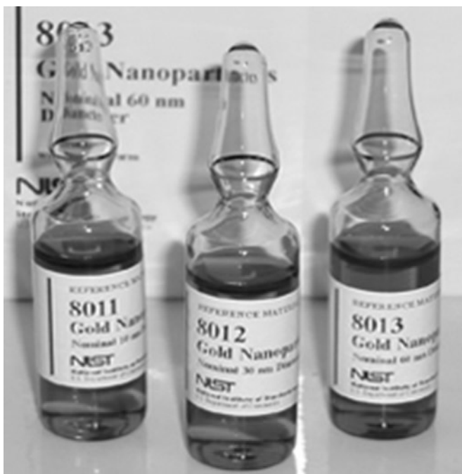
Figure 4. NIST certified-gold RMs with three different sizes—10 nm, RM 8011; 30 nm, RM 8012; and 60 nm, RM8013.
