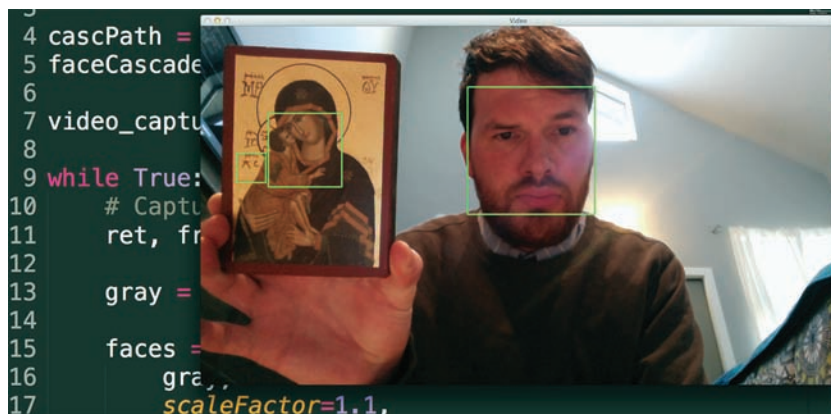
Figure 2.1. Real-time detection and tracking using OpenCV, Python, iSight, and a MacBook Pro. Image care of Jentery Sayers. Python script care of Shantnu Tiwari, modified by Jentery Sayers.
