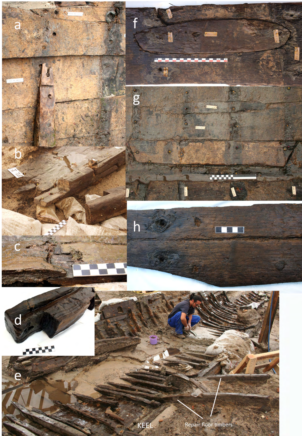
Figure 12.4. Examples of repairs from the Yenikapı shipwrecks: (a) Floor timber FL 44 from YK 14's hull. Note the caulked drilled holes next to the frame's location, which may be from an original frame, now removed; the timber's unique cross section and hook scarf are different from other frames on the ship. M. Jones, INA. (b) YK 24 Keel 3 timber, with the scarf for an endpost, Keel 4, which likely replaced more complex keyed hook scarfs normally used to join keel timbers. M. Jones, INA. (c) YK 14, PS 5-1A/5-2 scarf, at which an original plank piece was repaired with a worn, recycled timber. M. Jones, INA. (d) YK 11, end of the 'sternson,' recut from a keel timber (note the rabbet cut into the timber). R. Ingram, INA. (e) YK 4, replacement ash floor timbers in the midship area of the hull during excavation. M. Jones, INA. (f) YK 23, hull plank PS 4-1, with replacement piece PS 4-1A inserted in a rotten area (note the score mark and surface charring is missing on the repair piece). J. Čelebić, INA; (g) YK 14, replacement hull planks PS 2-1/1-2 and PS 3-1A, both recycled from a coak-built roundship similar to YK 14. M. Jones, INA. (h) A 'repair to a repair' (hull plank PS 6-2/1-4) from the hull of YK 14. A split in the plank (which was located at the turn of the bilge, and may have consequently been subject to more wear) was caulked. PS 6-2/1-4 was recycled from another ship (note the caulked treenail holes from its original use). The opposite end of the plank also had a repair piece installed into its scarf end (PS 6-2/5). Image by M. Jones, INA.
