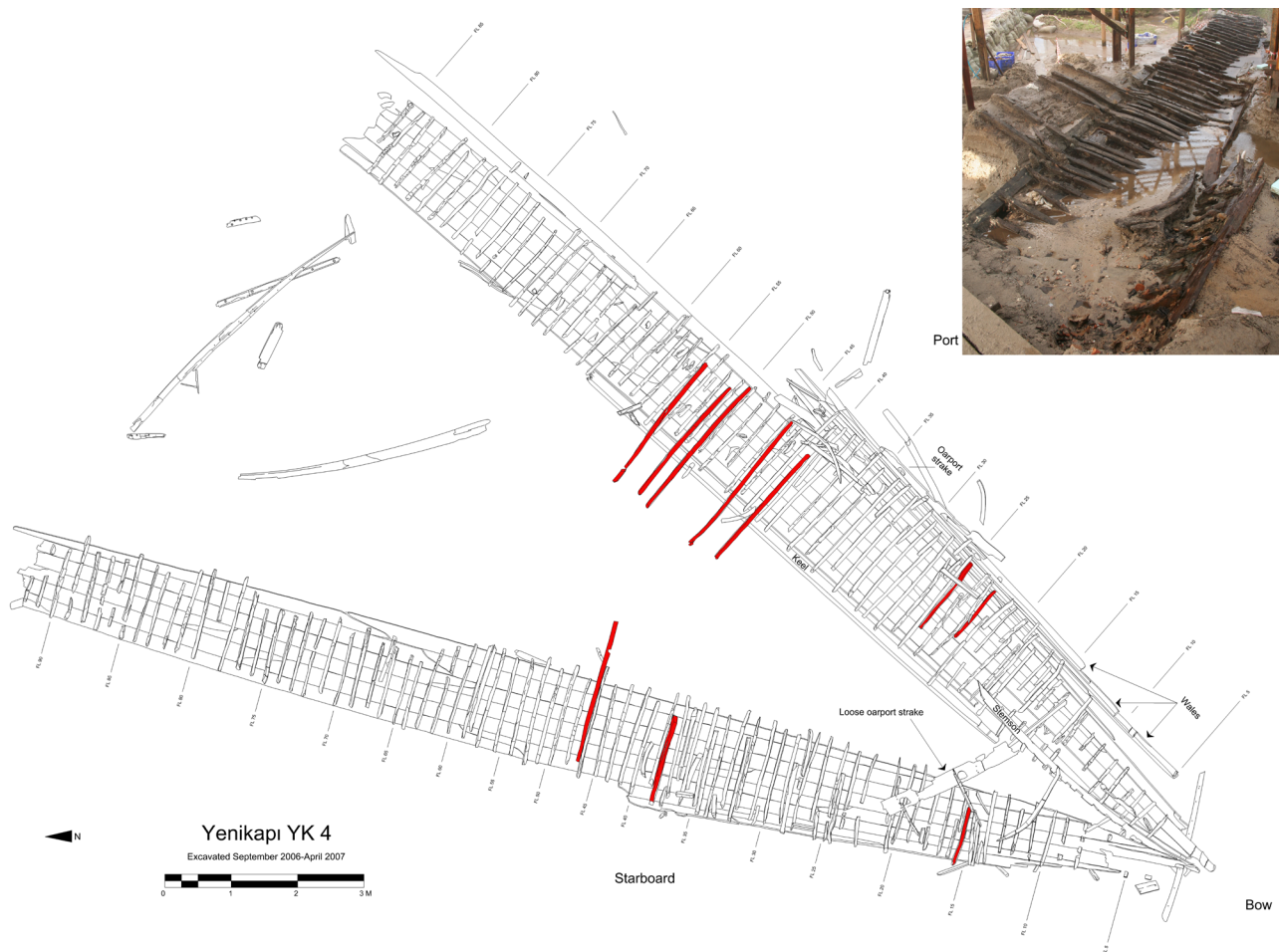
Figure 12.6. Site plan of YK 4, with identified repair frames shaded. Image by S. Matthews, INA; adapted by M. Jones.
