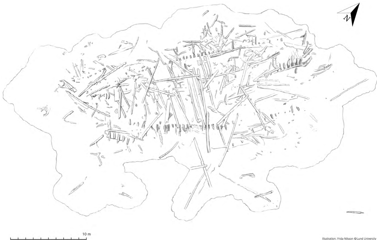
Figure 10.1. Site plan of Gribshunden shipwreck, derived from photogrammetric model. Illustration by Frida Nilsson, MediaTryck/Lund University.
