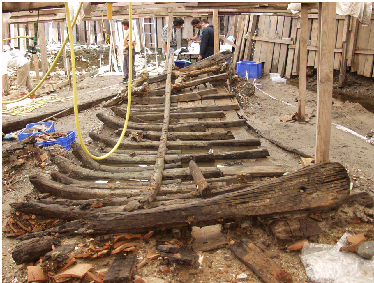
Figure 12.5. View of the preserved starboard side of YK 1, including strakes added during the overhaul of the ship, to the right. Copyright INA.
