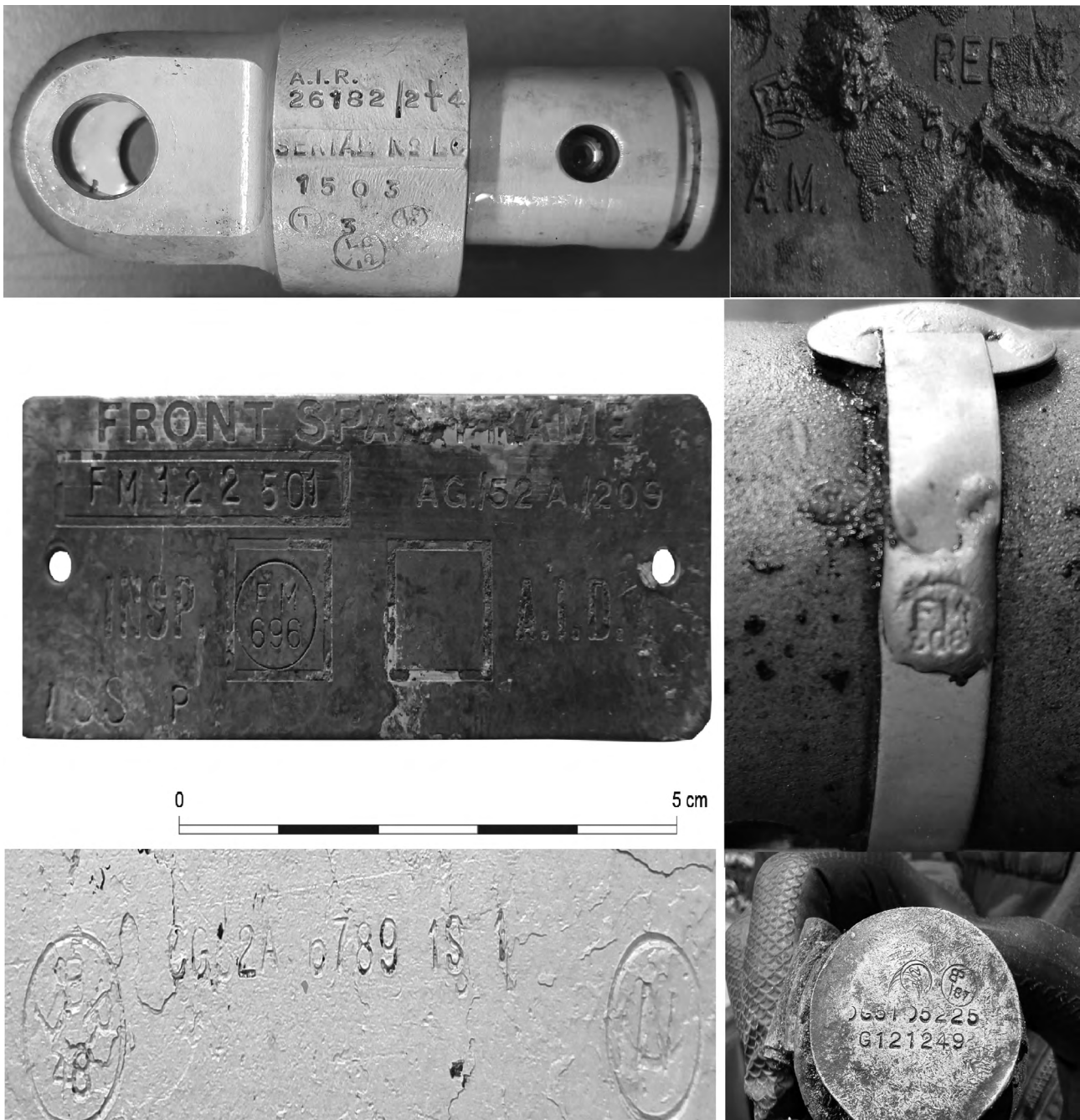
Figure 16.3. (Top left) AM embossed on electrical component. (Top right) Lockheed Precision Parts hydraulic component. (Centre left) Examples of Fairey inspection stamp with drawing and part numbers on front spar frame. (Centre right) Fairey Aviation brass hook and eye band with stamped solder. (Bottom left) Bolton Paul inspection stamp with issue one stamp next to drawing number. (Bottom right) Bolton Paul additional or super numary numbers. All images copyright Wessex Archaeology.
