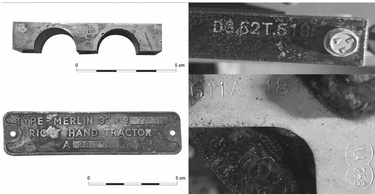
Figure 16.5. (Top left) Boulton and Paul stamped pipe clip. (Top right) Tufnol block for holding hydraulic pipes with ink stamp from the Solent wreck. (Bottom left) Rolls Royce Merlin 32 engine plate. (Bottom right) Westland quality control stamp and part drawing number on cockpit control arm. All images copyright Wessex Archaeology.
