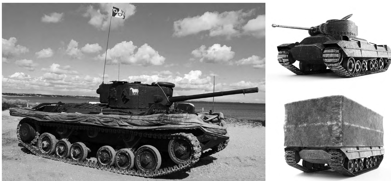
Figure 18.3. Top left: the last complete and working Valentine DD tank on Studland Beach in April 2019; top right: Valentine tank model (without canvas skirt); bottom right: Valentine DD model with deployed and fully raised canvas skirt. Image created by the Exercise Smash Development Team.
