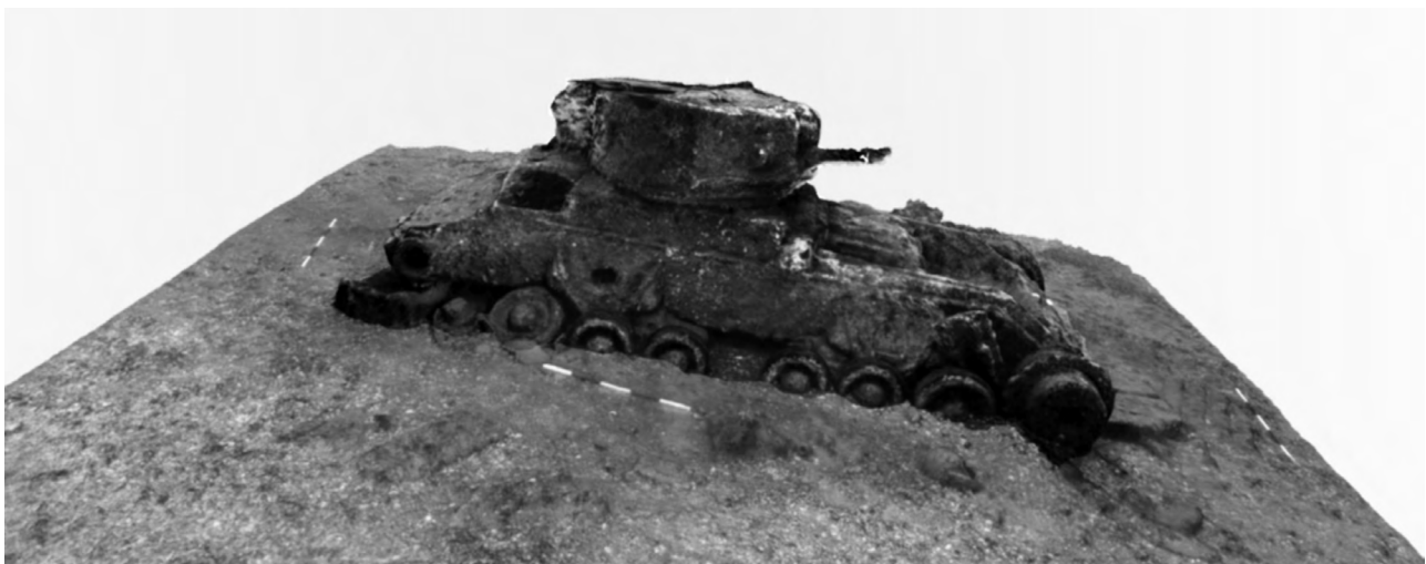
Figure 18.2. Underwater Photogrammetry of the complete (before the damage that occurred during 2022) ‘Tank 1’ (Valentine MK-IX DD) at the bottom of Studland Bay (3D model of 3.3 million vertices in 6.6 million triangles). Without a fixed survey grid on the tanks, the ‘rapid fire technique’ developed by Daniel Pascoe (Pascoe Archaeology Services) and Bournemouth University was used, employing a goPro6 camera with a 105 degree fisheye lens. Four one-meter scale bars were placed around the site, and then with the goPro’s time-lapse function, photos were automatically taken every second, with the diver slowly swimming over the site. The resulting photos were colour corrected using Adobe Photoshop and loaded into Agisoft Metashape where the images were further processed to mask out any undesirable features, such as the water column and fish, and to calibrate the lens to compensate for the wide angle which can cause issues with alignment. After processing and filtering with Metashape, the original photos were then used to create the texture-map. Finally, the model was scaled using the bars placed around the site during image acquisition before it was exported as a 3D object. Image created by the Exercise Smash Development Team.
