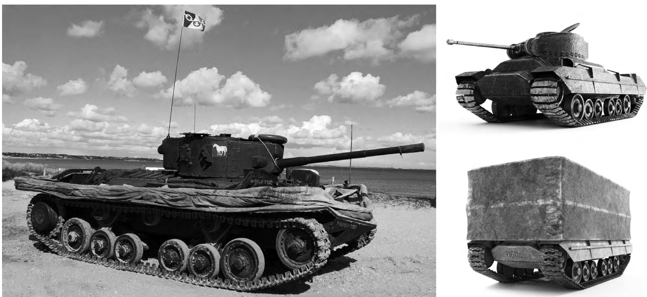
Figure 18.3. Top left: the last complete and working Valentine DD tank on Studland Beach in April 2019; top right: Valentine tank model (without canvas skirt); bottom right: Valentine DD model with deployed and fully raised canvas skirt. Image created by the Exercise Smash Development Team.
